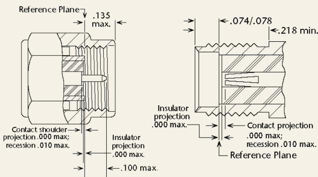
**SMA-RP (Reverse Polarity) Connectors**
