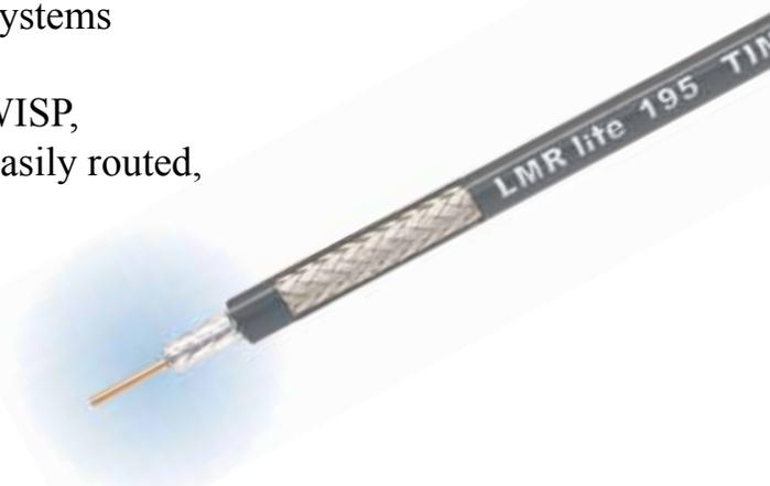
• **LMR-LW** is a lightweight low loss coaxial cable that employs an aluminum braid shield instead of the traditional tinned copper shield. LMR-LW has been designed and engineered with a combination of electrical, physical and mechanical properties that reduce weight and cost.
