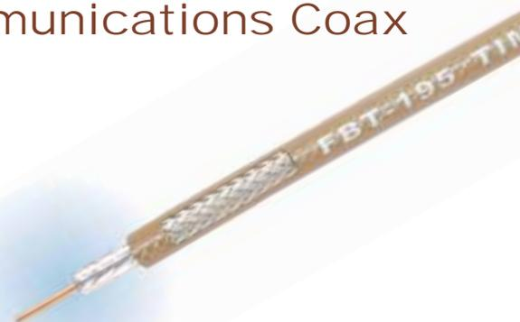
• **FBT™** is an indoor/outdoor highly fire retardant cable intended specifically for runs within and between base station cabinets. It is also applicable for return air handling plenums (e.g., dropped ceilings, raised floors). It has a UL/NEC rating of ‘CL2P’ for plenum applications.
